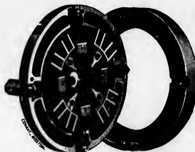
Inside view of Four-Jaw Chuck, showing the Screw and Pinions, the nut under the Jaw and the Gear which is loose in the Back Shell.
